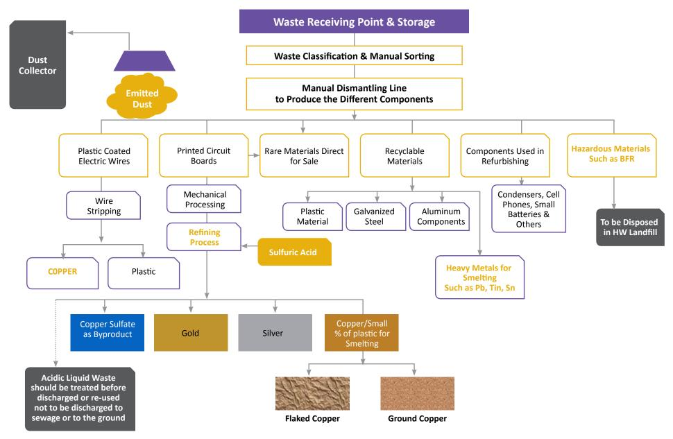
Figure 2: Process Flow Diagram of the Fractions Processing
