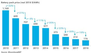
Figure 4: Li-ion battery pack price over time (volume-weighted average)  $^{\rm 10}$
