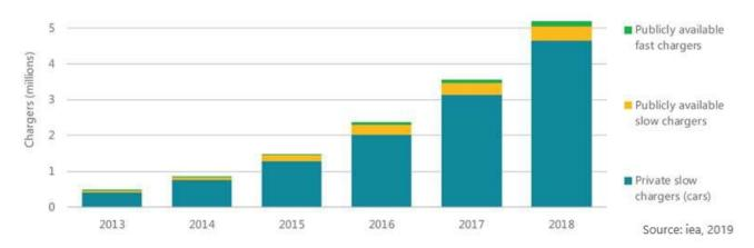
Figure 5: Global installation of electric LDV chargers, 2013-2018 indicating the vast majority being private slow chargers<sup>15</sup>.
